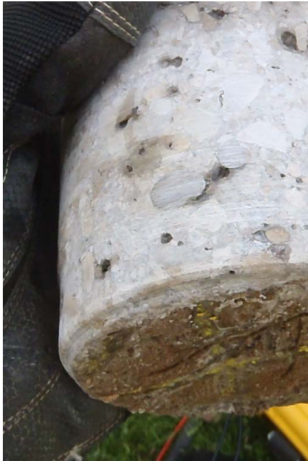
Concrete Cores Removed for Testing
