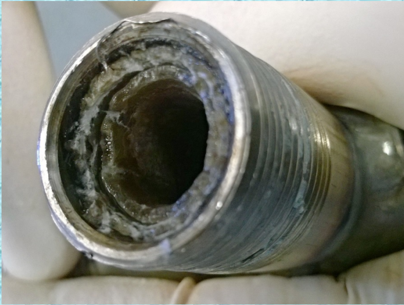
Before Periodic Cleaning in Dilute HCl
