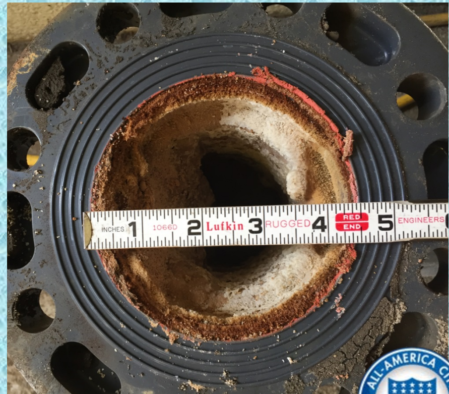
Chemical Line With "Potato Chips"
